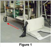
CAUTION! Ensure wheels are facing towards head end of the Trolley and brakes are applied before lowering!
