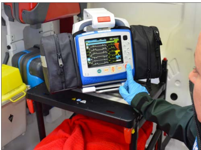
Zoll X-series monitor bracket mounted to PacRac+ using a swivel-mount SafeMount interface
